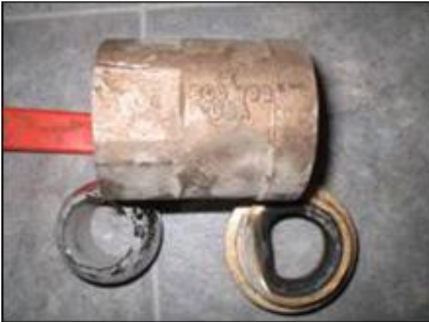
Above is a photo of the failed 250 psi valve. This valve was replaced with the appropriate 3000 psi valve
