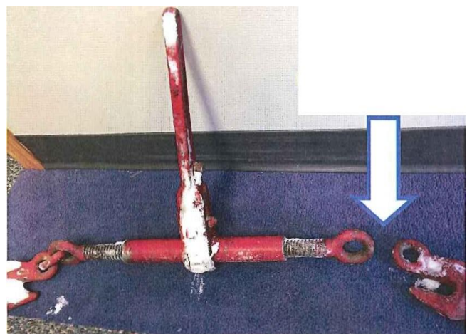
Broken Connection Link on Ratchet Boomer
