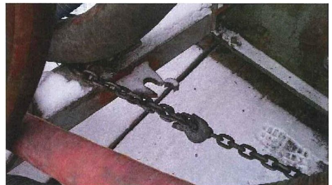
Location of where ratchet Boomer was attached to replace spreader bar
