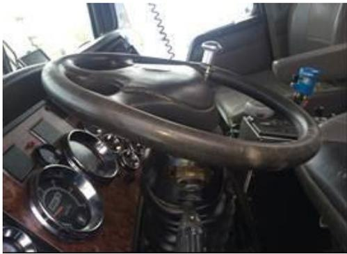
Damage to steering wheel from the impact of the driver's chest hitting it.
