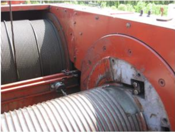
Figure 2 Drill Line Clamp In Place Position
