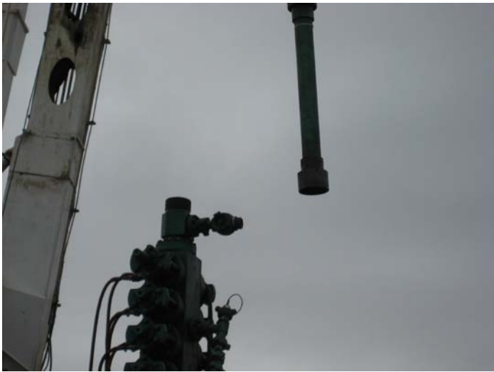
Image 2 is the approximate kick of the lubricator stack.
