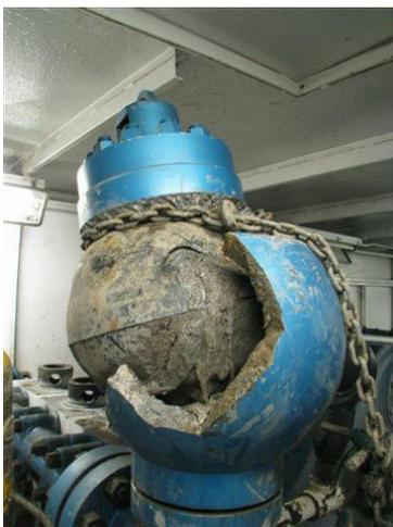
**Photograph #2 – A Typical Dampener Failure**
