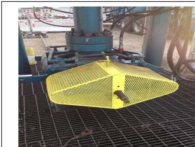
QRC Ram BOP hydraulic operator covered with engineered guard
