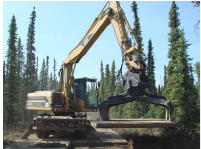
Photo #4 - Alternate lift systems can improve safety by eliminating rigging and terrain hazards
