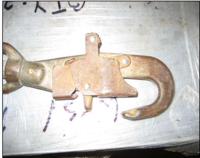
Photo of Damaged Double Latch Hook
