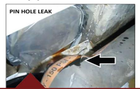
The source of the leak and the fluid streaming from it may be very small and not easily visible. It is important to only use the far end of a long object such as a piece of cardboard or wood in the suspected path of any fluid stream.
