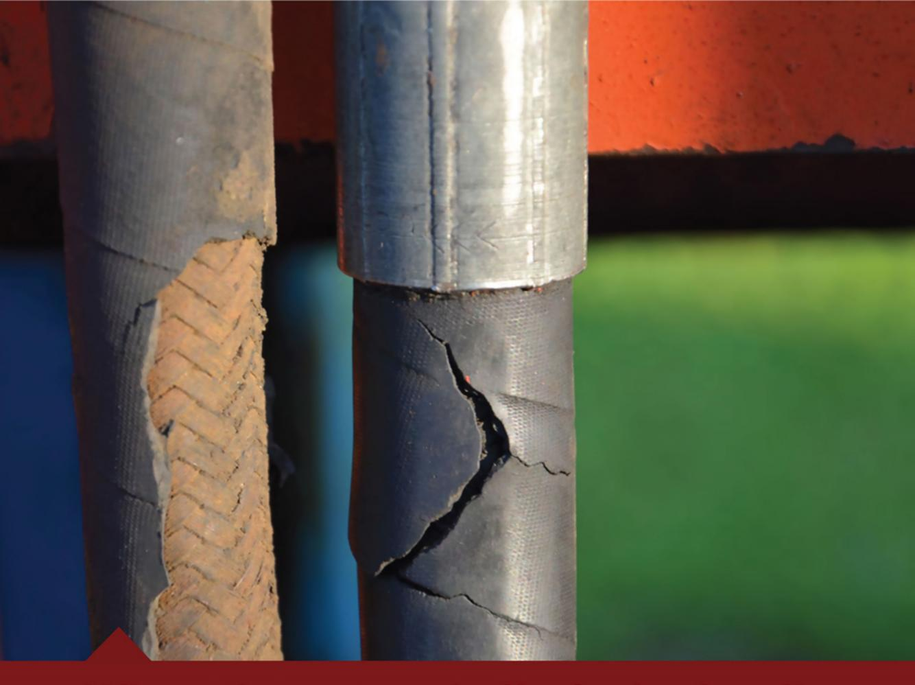
When the outer shell of a hydraulic hose is damaged the steel reinforcement wire begins to corrode. Hose rupture will soon occur.
