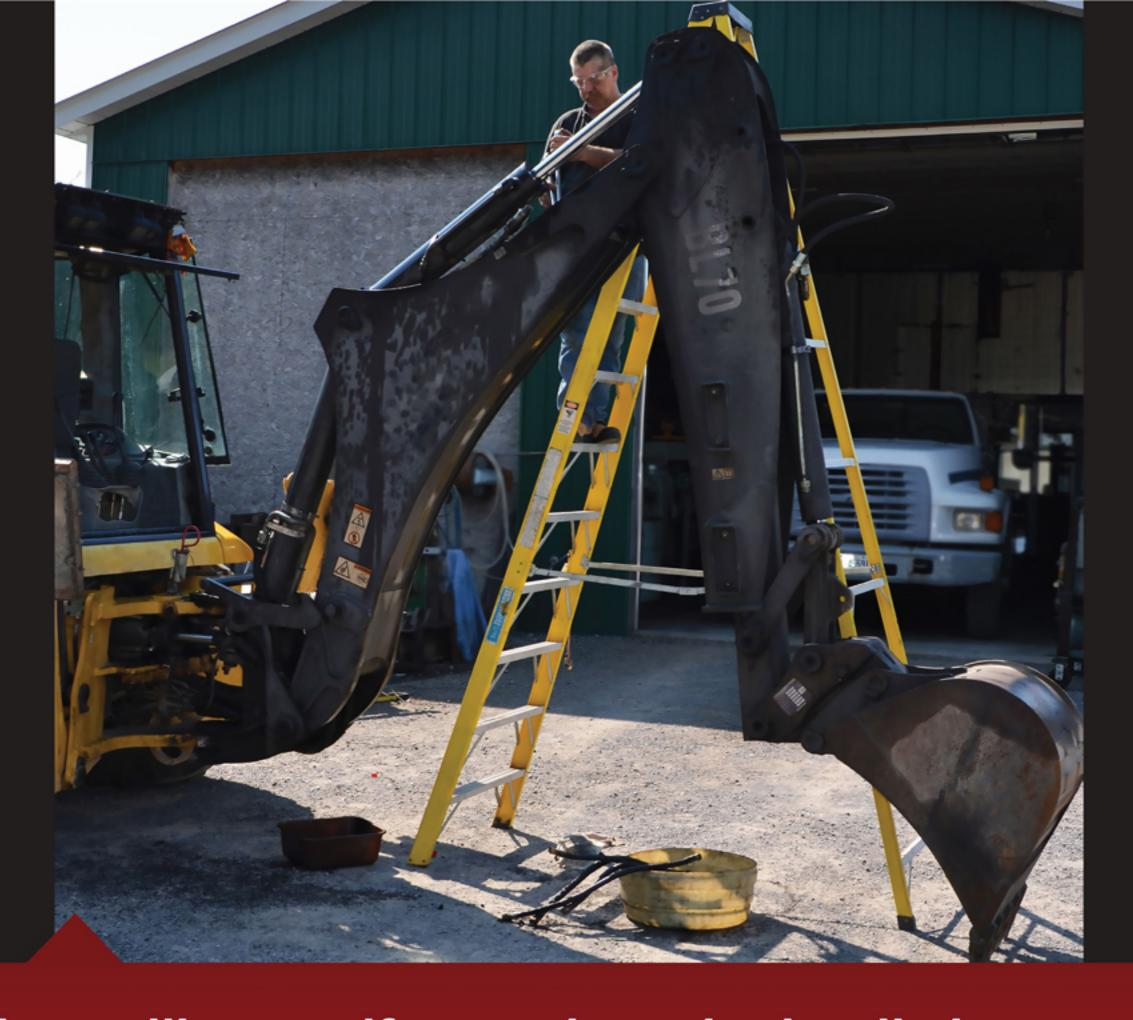
Injury will occur if removing a hydraulic hose sets equipment components into motion. Changing a specific hydraulic hose requires that an exact written procedure for specific component positioning be followed.
