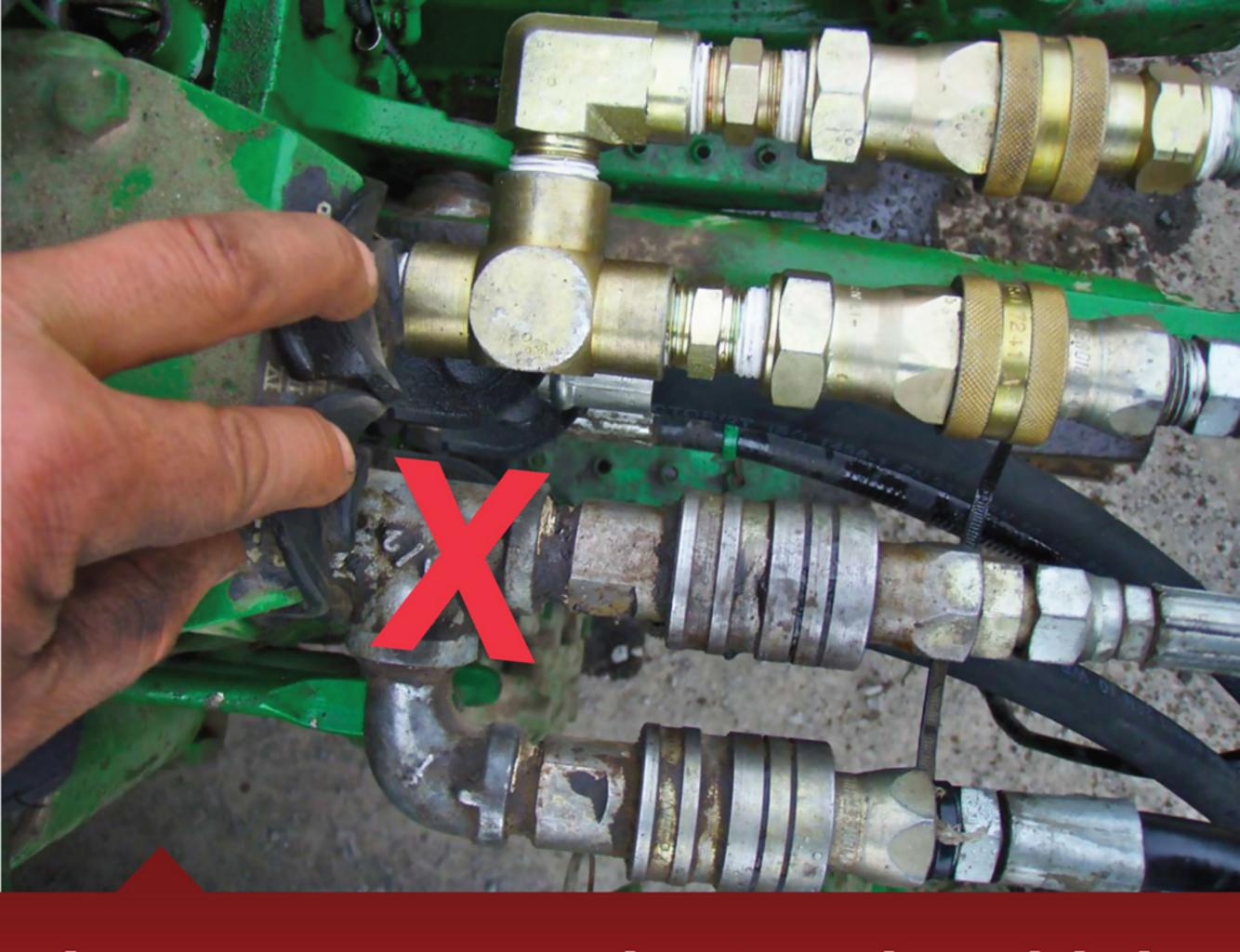
Low pressure adapters in a high pressure system is extremely hazardous.
